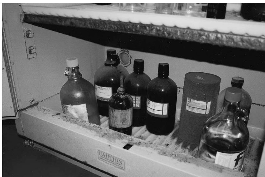
Figure 3. Incompatible chemical storage was discovered in this acid cabinet. Additionally, the integrity of the shelving has been seriously compromised by rust and corrosion. New shelves should be purchased, the cabinet should be thoroughly cleaned, and the laboratory supervisor must store these chemicals according to hazard category.
