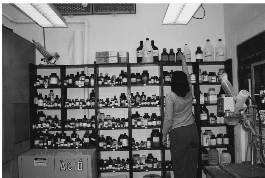
Figure 5. These chemicals are stored on shelving that exceeds five feet in height, creating a health risk and potential disaster for the laboratory worker. The person in the photograph is standing on a stool, reaching up to grasp a bottle containing a liquid material. If she loses her grasp on the bottle, or suddenly loses her balance and tries to grab the shelves to avoid falling, any number of bottles of chemicals could be broken. The laboratory worker could sustain chemical burns, cuts, and exposure to hazardous materials and fumes when incompatible chemicals are mixed during a catastrophic incident.
