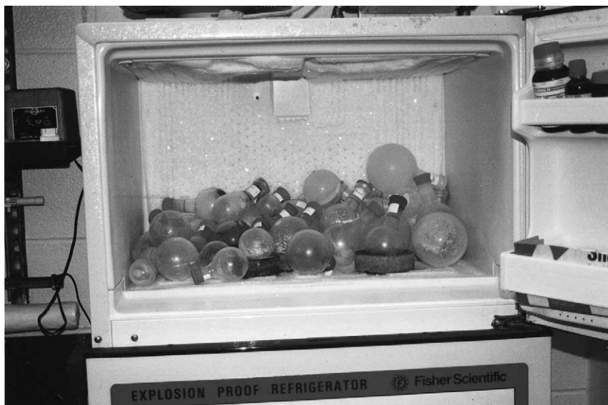
Figure 6. Refrigerators and freezers should be cleaned and defrosted on a regular basis. Missing labels should be replaced immediately and unneeded chemicals should be removed from the laboratory. The haphazardly stored and improperly labeled round bottom flasks in the photograph present an obvious safety risk to the laboratory workers (and the intrepid inspector) when the freezer door is opened.
