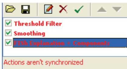
The detection method must always be the final action, but you can change the order of other filters in the Action pane.
