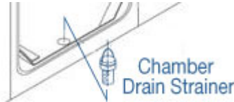
Figure 2. The location of chamber drain strainer.
