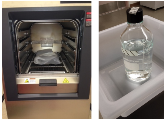
Figure 3. The position of sample loading and second container for liquid sample.
